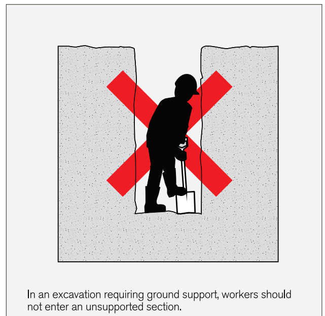
Figure 21 – In an excavation requiring ground support, workers should not enter an unsupported section
