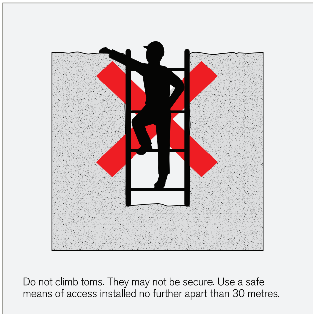
Figure 30 – Unsafe form of access
